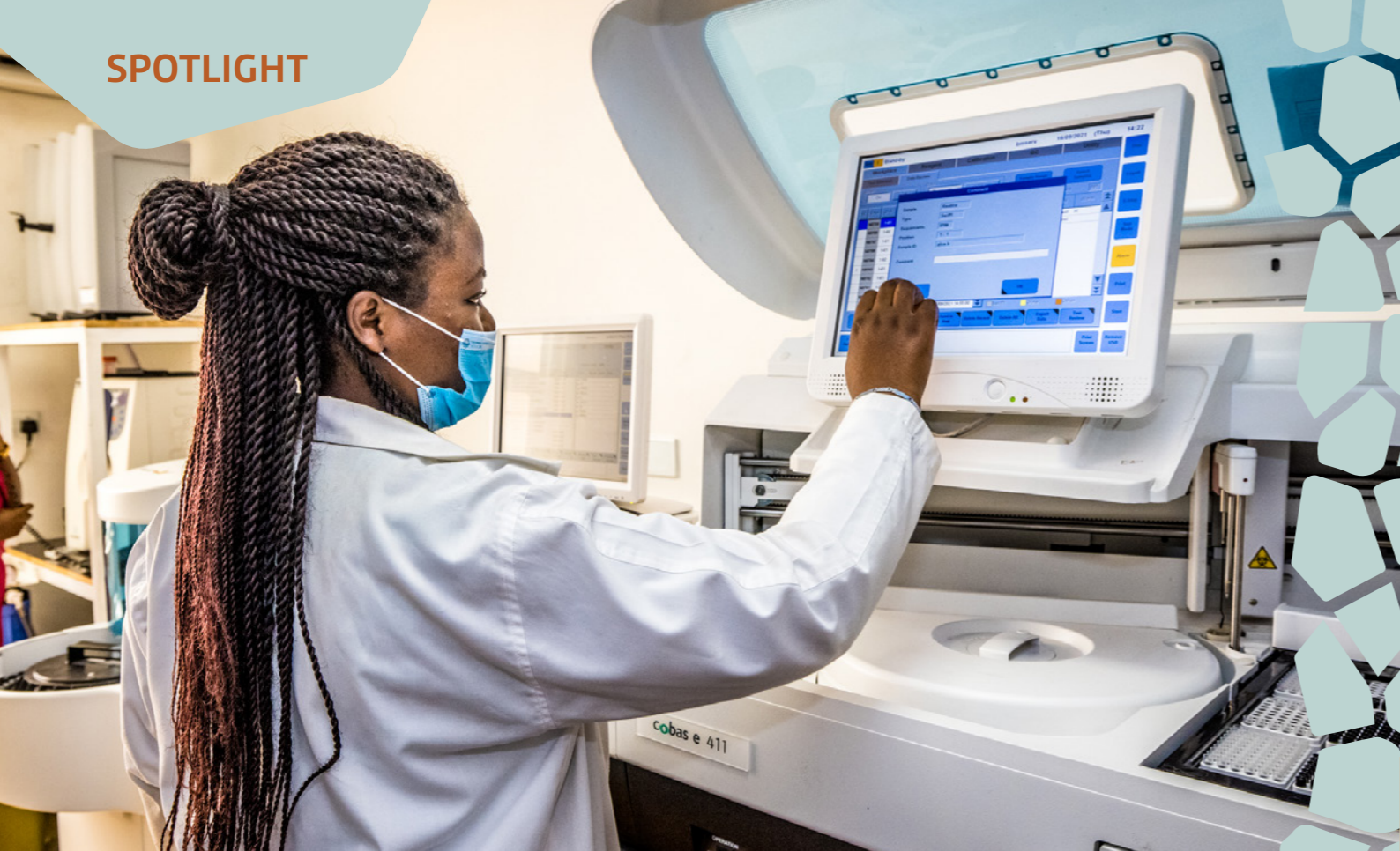
TMR staff operating the automatic immunological analyzer that is used to run automated biochemical tests for detecting cancer markers, diagnosing infectious diseases, cardiac analysis, and other testing.
